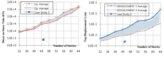
Fig. 22 Average Values of Shear Forces for .Tube-in-Tube of Fig.3
