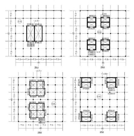
Fig. 1 Structural Systems used in Core (Shear Wall) Case
