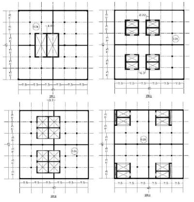
Fig. 2Structural Systems used in Core (Shear Wall) with Outrigger.
