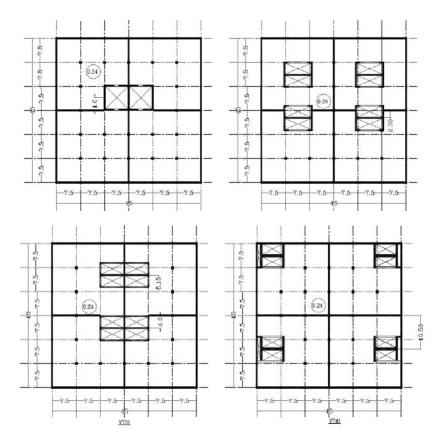
Fig. 4(Cont.) Structural Systems used in Tube-in-Tube with Outrigger.
