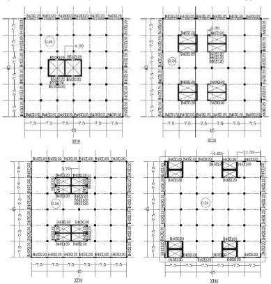
Fig. 3Structural Systems used in Tube-in-Tube.
