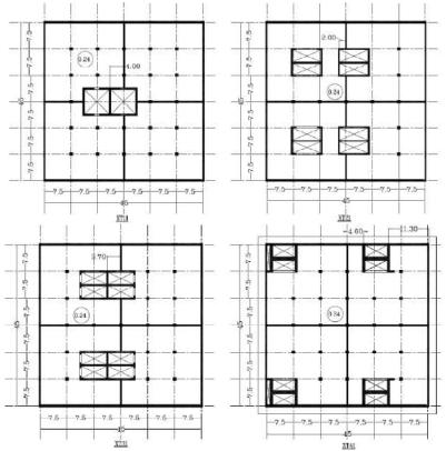
Fig. 4Structural Systems used in Tube-in-Tube with Outrigger.
