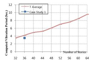
Fig. 11 Average Values for Vibration Periods for Shear Walls of Fig.1.
