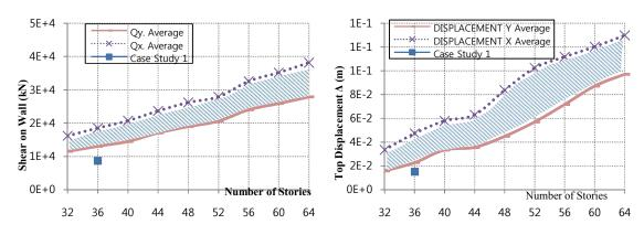
Fig. 8Average Shear Forces for Shear Walls of Fig.1. Fig. 9Average Values of Top Displacements for Shear Walls of Fig.1.
