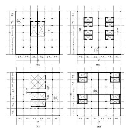
Fig. 2 (Cont.)Structural Systems used in Core (Shear Wall) with Outrigger.
