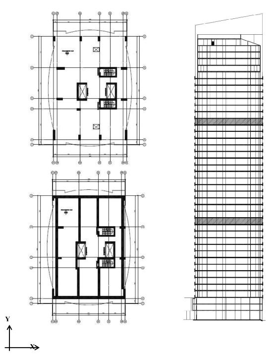
Fig. 19Structural System for Case Study (2)of Shear Wall with Outriggers.
