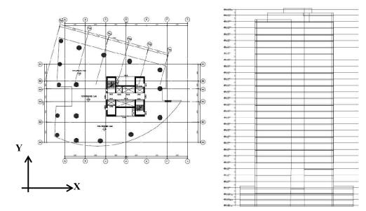
Fig. 12Structural System for Case Study (1)ofShear Walls.
