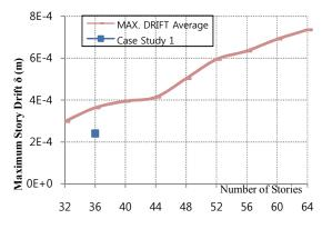
Fig. 10Average Drifts Values for Shear Walls of Fig.1.
