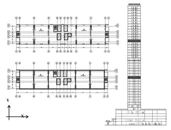
Fig. 33Structural System for Case Study (4)of Tube-in-TubeCase.
